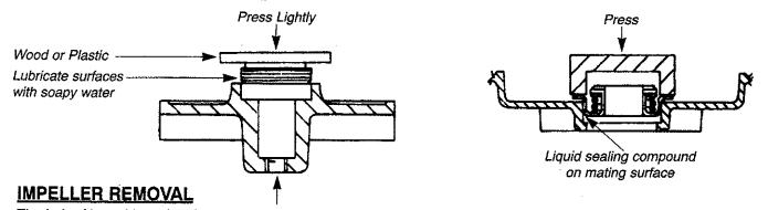
The hub of keyed impellers is tapped M12. Remove the centre bolt which is either 5/16" UNF, M8 or 3/8" UNF depending on the shaft. If the impeller is tight on the shaft due to rust, proceed as follows: Insert a short grub screw, with the same thread as the centre bolt, to the end of the shaft. Screw an M12 bolt into the hub of the impeller. This will act as a puller.
